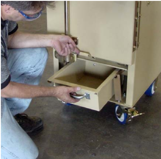
Tool-less, quick-release dust drawer for removal of the captured powdered sweetener.
