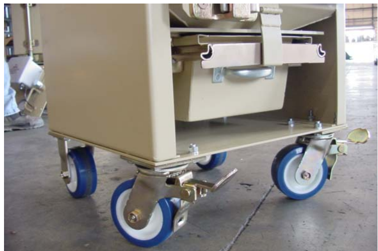
Heavy duty food grade casters provided the portability that Wrigley wanted in order to configure machinery layout for changing production schedules and requirements.
