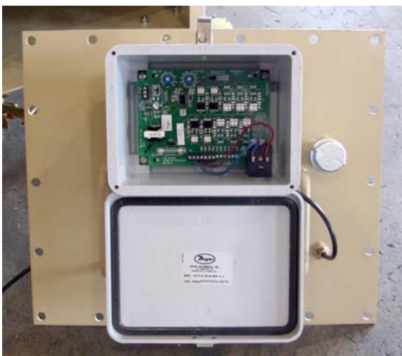
Optional automatic timer cleaning system - Wrigley decided to use their own central computer PLC to actuate the cleaning components.
